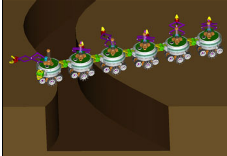
Figure 2: A swarm-bot made of several assembled s-bots passing a fosse.
