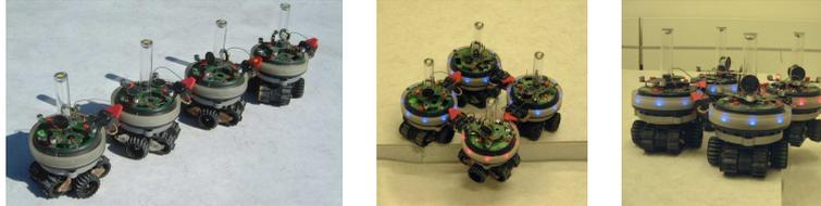
**Figure 1.5.** Left: four real *s-bots* forming a linear *swarm-bot*. Centre and Right: four *s-bots* coordinately move and avoid falling. Notice that one *s-bot* is suspended out of the border of the arena, and the physical connections among *s-bots* provide support.
