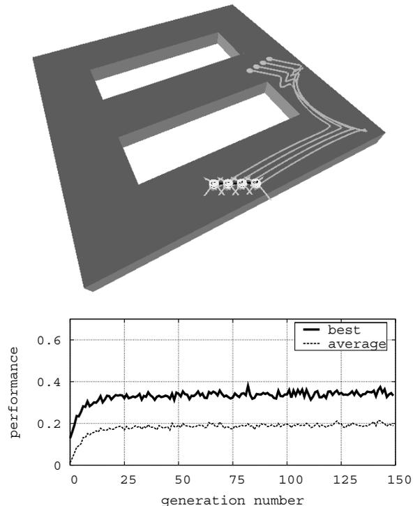
Figure 3. The hole avoidance task. Top: The picture shows the arena used, which presents open borders and contains two large rectangular holes. A *swarm-bot* composed of four linearly connected *s-bots* is shown, along with their trajectories while avoiding holes. Bottom: The average fitness of the best individual in the 10 replications of the experiments and the average fitness of the population are plotted against the generation number.
