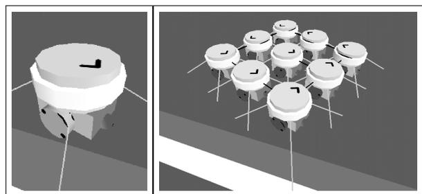
Figure 2. The simulation model. Left: a simulated *s-bot*, where many details not relevant for our experiments have been omitted. Right: a *swarm-bot* formed by 9 *s-bots* in a square formation.
