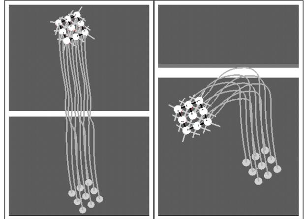
Figure 5. Trajectories drawn by a *swarm-bot* composed of 9 *s-bots* in a square formation. Left: the *swarm-bot* is able to pass over a 10 cm wide trough. Right: the *swarm-bot* avoids a 20 cm wide trough, which could be too large to be bridged.
