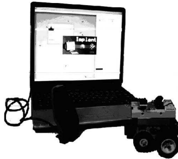
Fig. 3. The transfer of the control system (an Artificial Neural Network) from the Digital Environment to the real Lego MindStorms robot, through the infrared port.
