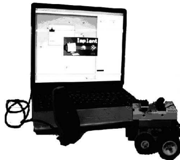
Figure 3: The transfer of the control system (an Artificial Neural Network) from the Digital Environment to the real Lego MindStorms robot, through the infrared port.
