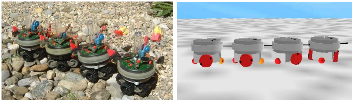
Figure 5. Left: Four robots assembled into a linear structure. Right: A simplified simulation of the robots described in the left part of the figure based on Vortex TM libraries.
