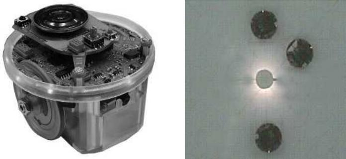
**Fig. 1** Left: The e-puck robot developed at the Swiss Federal Institute of Technology in Lausanne (EPFL) (Mondada and Bonani, 2007). Right: A close up view of the environment with the light bulb in the centre and three robots.
