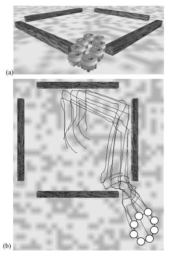
Figure 12: (a) A swarm-bot deforms its structure and succeeds in exiting a walled arena with four narrow passages. (b) The traces left by a swarm-bot engaged in exiting the arena.
