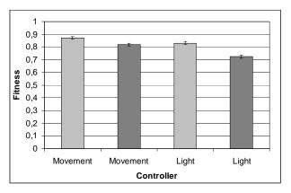
Figure 13: Performance (y-axis) of the evolved neural-network controller (light grey bars) and of the double motor schema-based controller (dark grey bars) in a coordinated motion test ("Movement") and in a light approaching test ("Light"). Each histogram bar reports the average performance and the standard error of the controllers obtained in 100 trials. The data relative to the evolved neural controllers are those produced by the experiments described in detail in Baldassarre et al. (2004).
