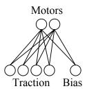
Figure 5: The neural controller of each robot consisted of a twolayer neural network with five input neurons, encoding the direction and intensity of traction plus a bias signal, and two output neurons, encoding the desired speed of the wheel motors.
