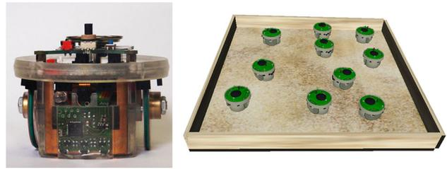
**Fig. 1** The experimental set up. *Left* the e-puck robot. *Right* the arena with ten simulated robots
