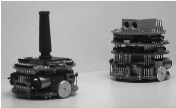
Figure 1: **Right:** The Predator is equipped with the vision module (1D-array of photo-receptors, visual angle of  $36^\circ$ ). **Left:** The Prey has a black protuberance which can be detected by the predator everywhere in the environment, but its maximum speed is twice that of the predator. Both Predator and Prey are equipped with 8 Infrared proximity sensors (max detection range was 3 cm in our environment). Evolutionary runs have been conducted in simulation.
