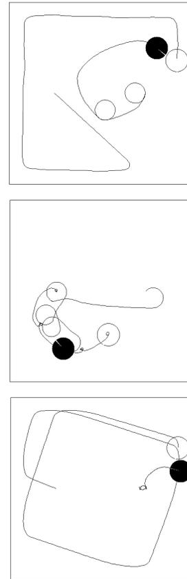
Figure 4: Behaviors of *genetically-determined controllers*. Black disk is predator, white is prey. **Top**. Generation 20: The predator has developed good visual tracking strategies. The prey is a wall-follower with obstacle avoidance. **Center**. Generation 70: The prey turns on place quickly backing whenever the predator attacks. **Bottom**. Generation 90. The predator develops a “spider-strategy” slowly backing against a wall and waiting for the fast-approaching prey.
