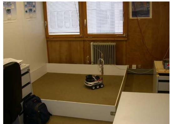
Figure 61.14: A mobile robot with pan-tilt camera is asked to move within the walled arena in the office environment.
