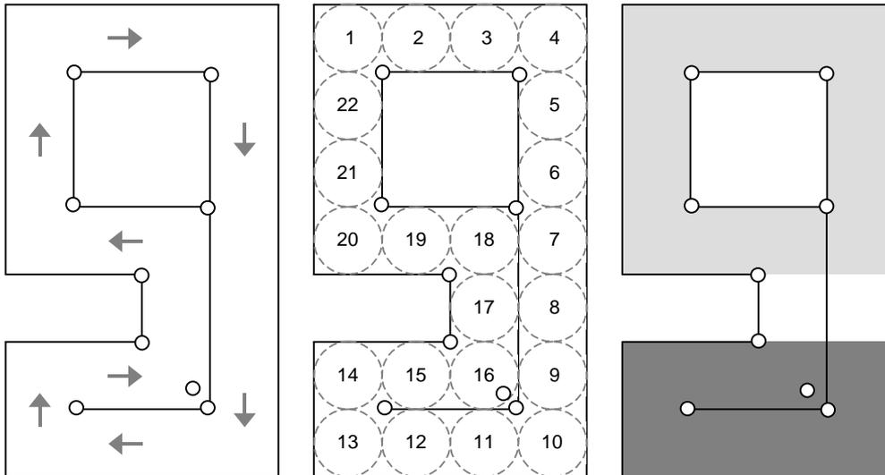
**Figure 7.** **Left:** The environment consists of a loopy corridor of 40x70 cm. Lines represent walls. Circles represent cylindrical objects. Arrows represent the starting positions and orientations in which the robot is placed at the beginning of each trial. **Center:** The environment is divided into 22 idealized regions placed along the corridor clockwise. **Right:** The environment is ideally divided into two rooms indicated with light and dark grey colours.
