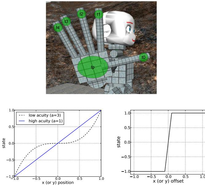
Fig. 4: Top: Location of the touch sensors in the robot’s hand. Bottom Left: State assumed by the first two sight sensors for different positions of the colored blob field of view. The dashed and full lines indicate how the state varies with low and high acuity vision respectively. Bottom Right: State assumed by the two sight sensors on the basis of the offset between the position of the ball and the position of the hand in the robot’s view field.
