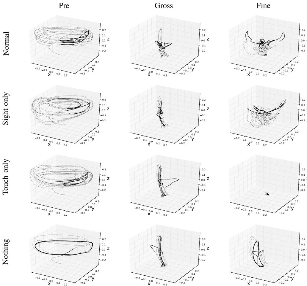
Fig. 8: Trajectories of the robot’s hand observed during post-evaluation analysis in which the robots have been deprived of tactile and/or visual sensory information. Data collected for one trial on the best robot of the best replication at the end of the pre-, gross-, and fine-reaching phases.
