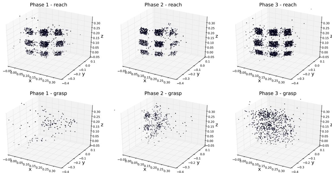
Fig. 7: Spatial distribution of successful reaches (upper row) and grasps (lower row) at the end of the pre-, gross-, and fine-reaching phases. Data obtained during a post-evaluation analysis in which the 5 best robots of each of the 10 replications of each phase has been tested for 45 trials, during which the position of the target objects has been systematically varied so to cover all possible target positions.
