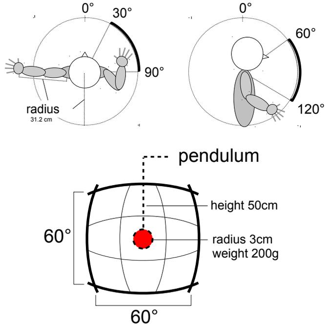
Fig. 2: The thick line in the three pictures shows the portion of the spherical surface in which the ball can be placed. To ensure a good spatial distribution over space of the target objects, the surface is virtually divided into 9 sectors.
