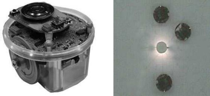
**Fig. 1.1.** Left: The e-puck robot developed at the EPFL in Lausanne, Switzerland (Mondada and Bonani 2007). Right: A close up view of the environment with the light bulb in the centre and three robots.
