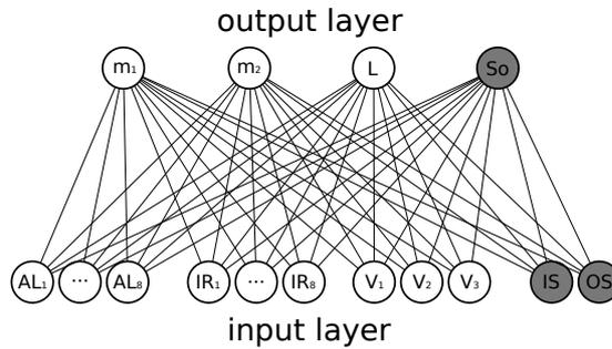
**Fig. 1.3.** The architecture of the neural controller. Note that gray neurons refers to virtual actuator/sensors not present in the physical robot, but implemented through the wireless bluetooth interface. Neurons “AL” are used in the experiment  $E_I$  only, while the other neurons are common to both setups.
