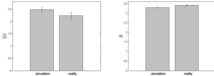
**Fig. 1.7.** Average mutual information ( $\widehat{MI}$ ) and entropy ( $\widehat{H}$ ) computed by testing the best evolved controller of run 9 of experiment  $E_t$  in simulation and in reality for 20 trials of 2000 cycles. During the tests in hardware, the robots were situated in the same randomly generated positions and orientations that were used for the tests in simulation.
