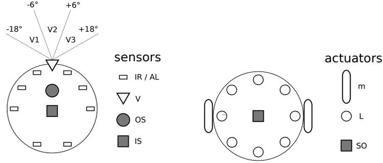
**Fig. 1.2.** Robot sensors and actuators. Left: sensors “IR” ( 8 infrared sensors), “AL” ( 8 light sensors), “V” ( 3 fields of view from pre-processed camera data), “IS” (average group signal), “OS” (own signal). Right: actuators “m” (wheel velocity and direction), “L” (leds ring on/off), “SO” (signal). Note that gray symbols refer to virtual actuators/sensors not present in the physical robot, but implemented through the wireless bluetooth interface.
