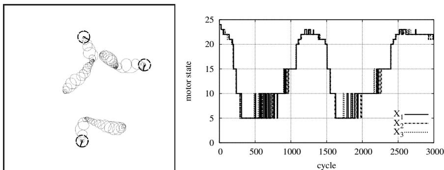
**Fig. 1.10.** Left: Trajectories of the robots produced by the best evolved controller in run 8 of experiment  $E_d$ . Right: The motor states of the three robots are plotted against the number of cycles.
