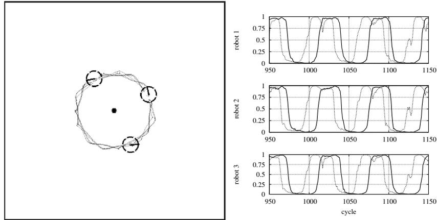
**Fig. 1.4.** Analysis of the behaviour produced by the best evolved controller in run 16 of experiment  $E_i$ . Left: trajectories of the robots. Right: activation of the motor neurons of each robot, plotted from cycle 950 to cycle 1150 to highlight the periodic motion of the robots. The solid and dotted lines indicate respectively the left and right motor neurons.
