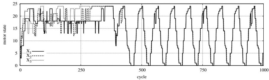
**Fig. 1.5.** The motor states of the three robots—computed using eq. (1.11)—are plotted against the number of cycles. Notice the initial coordination phase, followed by synchronised movements.
