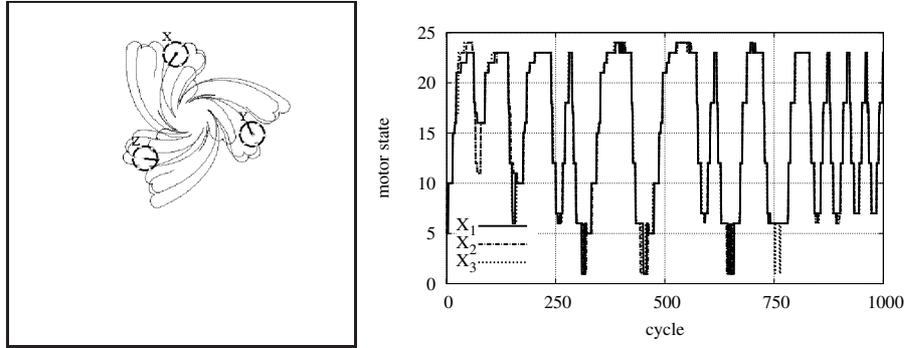
**Fig. 1.8.** Left: Trajectories of the robots produced by the best evolved controller in run 6 of experiment  $E_d$ . Right: The motor states of the three robots are plotted against the number of cycles.
