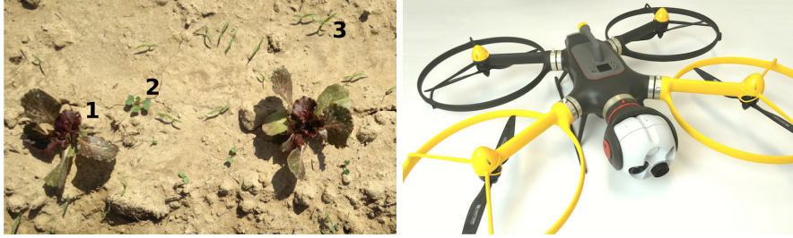
Fig. 1 Left: Young lettuce crop (1) with two types of surfacing weeds (2 and 3). In SAGA, we will perform object detection or semantic segmentation on images like this. Right: a close-up view of the PrecisionScout, the UAV produced by Avular B.V. and exploited within the SAGA experiment.
